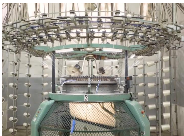
Figure 4.3: Circular knitting machine Figure 4.4: Fabric roll
